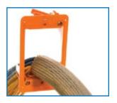
Install the sleeving over your wire bundle. Try to closely match the sleeving diameter to your bundle diameter so the bundle is fairly tightly managed. Leave about  $2^{\prime\prime}$ of additional length to put through to the other side of the finished assembly.
